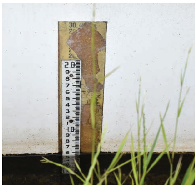
A staff gage reading at a stage of approximately 0.56 ft. The stage correlates to a flow rate using a table.
